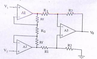
If  $R_G=5$  k $\Omega$ ,  $R_F=10$  k $\Omega$ ,  $R_1=1$  k $\Omega$ ,  $R_2=2$  k $\Omega$ . What is the voltage if  $V_{in}=V_2-V_1=1mV$ ? output
