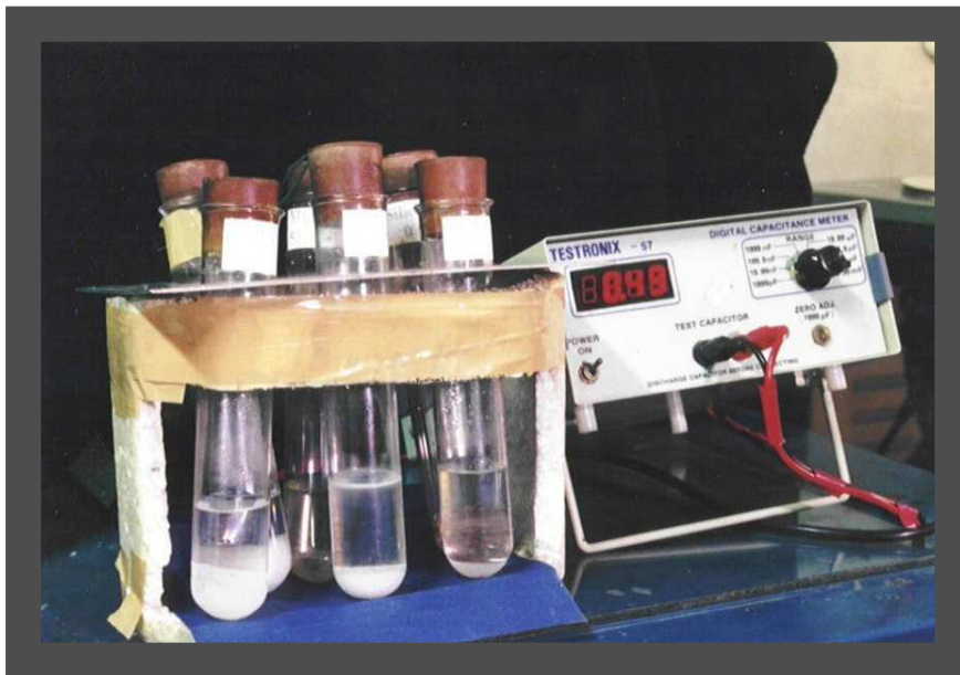
Plate-III: Step static RH measurement set up
