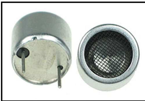
Fig.2.2 (a) Encapsulated ultrasonic sensor
