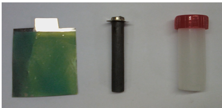
Fig. 6 (f) Photographs of potentiostatically deposited \text{Co}_{1-x}\text{Ni}_x LDHs thin films on to flexible stainless steel substrates having area 20 \text{ cm}^2
