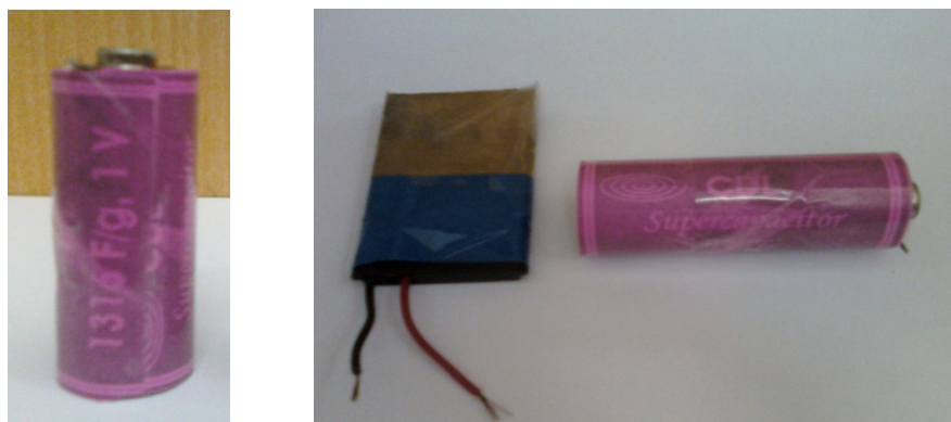
Fig. 6 (i) Final photographs of supercapacitive model based on potentiostatically deposited \text{Co}_{1-x}\text{Ni}_x LDHs electrodes
