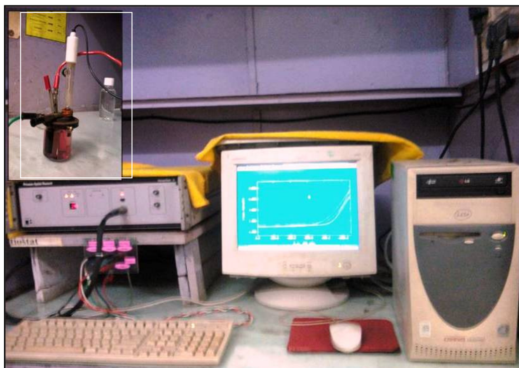
Fig. 3.2: Actual experimental setup for deposition of \text{Co}_{1-x}\text{Ni}_x LDHs thin films along with electrochemical cell.
