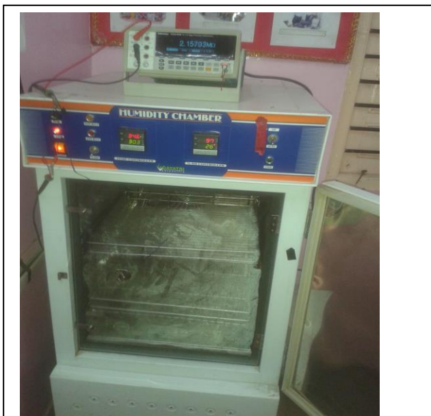
Figure 3.B.2: Experimental arrangement for measurement of humidity dependent characteristics of the composition under investigation.
