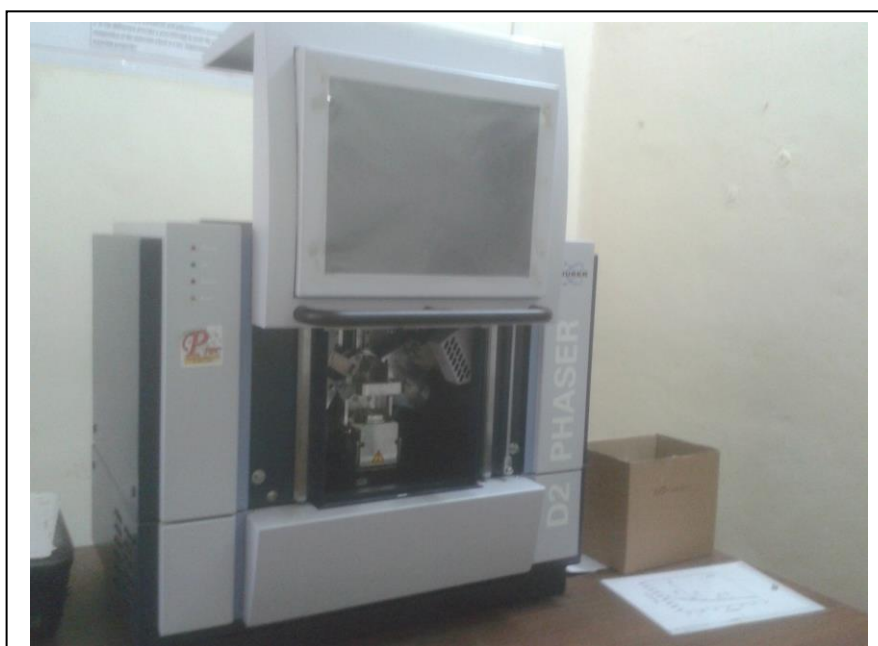
Figure 2.B.1: Experimental set up for X-Ray Powder Diffraction X-ray diffractometer Bruker AXE Analytical Instrument Pvt. Ltd. Germany, model D2 Phaser.
