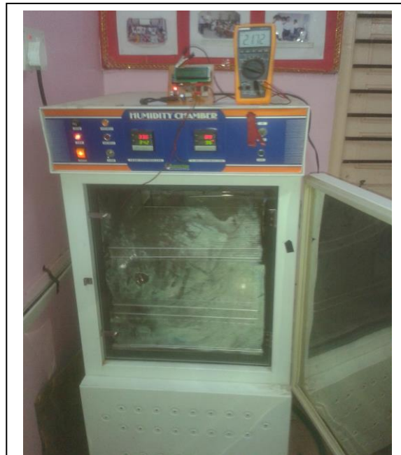
Figure 5.2: Experimental set up to determine the range of variation of observed emf ( V_{RH} ) for humidity varying from normal room condition to the condensation of the water molecules.
