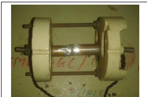
Figure 3.A.2: The Schematic of Electrode designed to measure resistance of the compositions using two probe methods.
